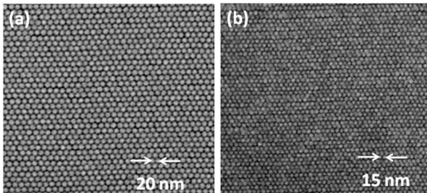
Scanning electron microscopy images of magnetic bits at densities of (a) 1.9 Terabit/in<sup>2</sup> and (b) 3.3 Terabit/in<sup>2</sup> formed after depositing Co/Pd multilayers onto resist structures.
